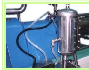
**Cooling System For Mechanical Seal**
